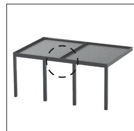
When column usage is not desired at module connection points, support columns should be used on both sides of the joint, no more than 1 meter apart. 30x70 mm steel box profiles are slid into the beams and joined end-to-end.
