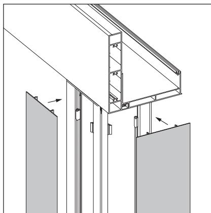
Column cover connections are the same as those used on corner columns. However, only flat cover profiles are used on support columns.
